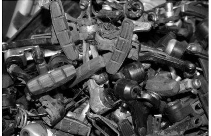
The bikes are donations: old bikes, unwanted bicycles that have been sitting in hallways, sheds and garages. The Bike Project gladly accepts any bike, and strips it down to its frame and fork, putting the parts into the part buckets, after cleaning and examining them. For every four bikes they get, they can make three working bikes, with some spare parts. Any broken frames go to the people who build festival bikes to be welded into another strange human powered contraption.
